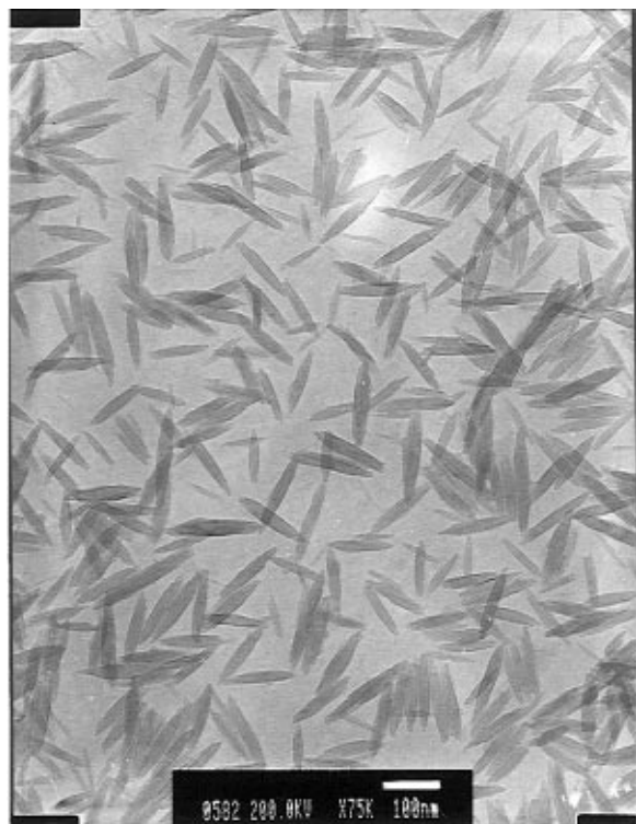
Figure 3. Transmission electron micrograph of a BBL/PPy blend sample having a PPy volume fraction of 0.10 and a conductivity of 1 S/cm. The white bar scale is 100 nm.
